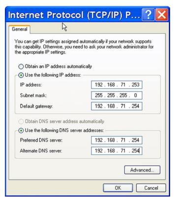
Temporary Network Configuration for Connection with Firewall Defaults - Windows
